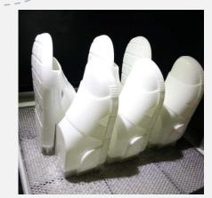
3D printing shoe mold for batch production
