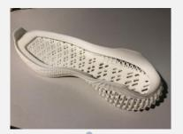
3D printing shoe model for testing appearance and structure (sla hard material)
