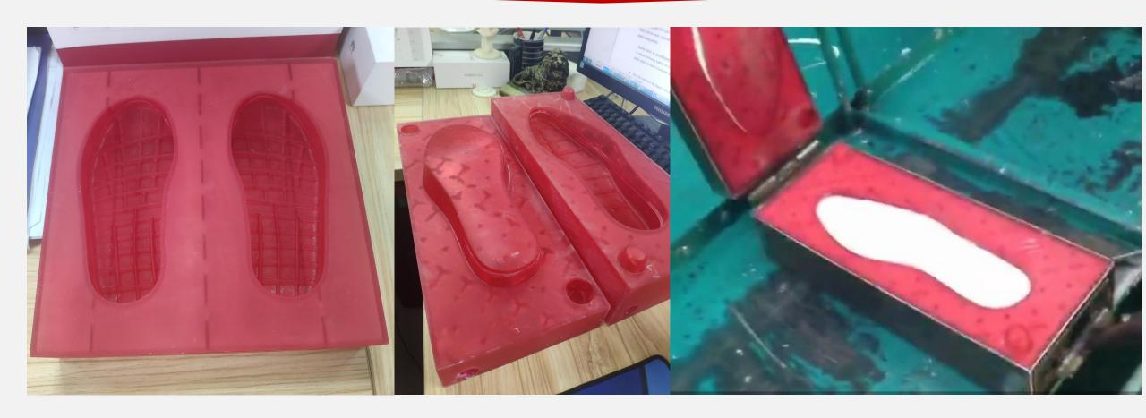
The molds produced by 3D printing can be directly used in the production of finished shoe soles. It can be used for plastic injection, PU and cold-pressed insole molds. It is not suitable for hot-pressed rubber, molded EVA and injection EVA. Generally, it can produce 10000 pairs of parts.
