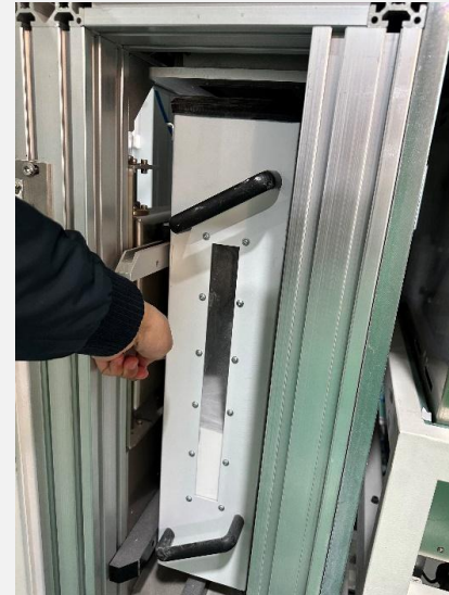
Lift the handle of the powder overflow cylinder and make the powder overflow cylinder move down
