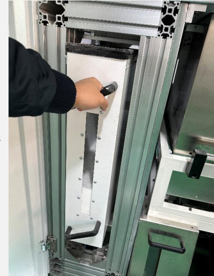
Pull out the spill tank forward
